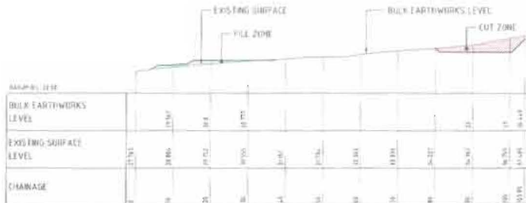
BULK EARTHWORKS CROSS SECTION 3 SCALE @ 1:100 HORIZONTAL 1:100 VERTICAL
