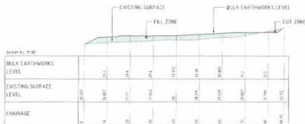
BULK EARTHWORKS CROSS SECTION 2 SCALE @ 1:100 HORIZONTAL 1:100 VERTICAL
