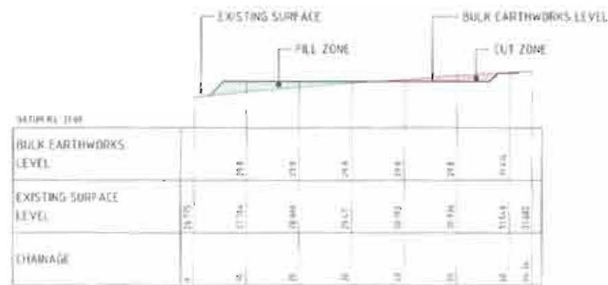
BULK EARTHWORKS CROSS SECTION 1 SCALE @ 1:100 HORIZONTAL 1:100 VERTICAL
